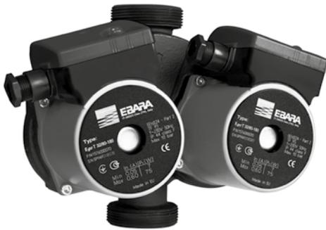
High performance wet-rotor circulation pump with threaded connection, motor with permanent magnets and built-in electronic controller.
